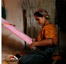
A horizontal loom in which one of two beams holding the warp yarn is attached to a strap that passes across the weaver's back.
